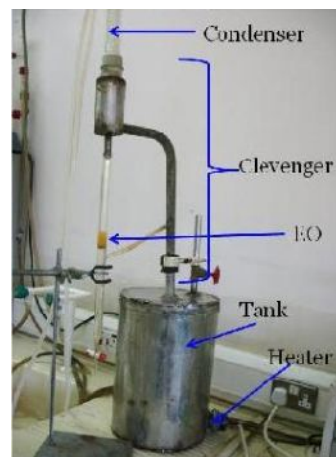
Figure 1: Essential Oil steam distillation with clavenger for oil separation.
