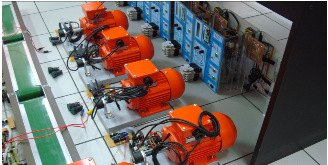
Figure 7: AC motors and conveyor belts in one of the laboratories ready to be used with the designed converters and controllers in a workshop
