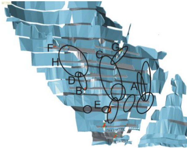
17 Three-dimensional numerical modelling results for F zone showing high stress concentrations at offsets (Suorinen et al., 2007)
