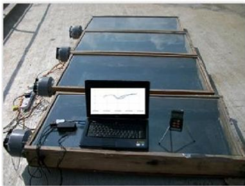
Figure 11: General experimental setup of flat plate solar collector
