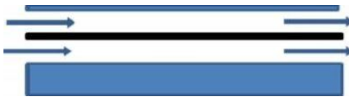
Figure 3(b): Double duct parallel flow
